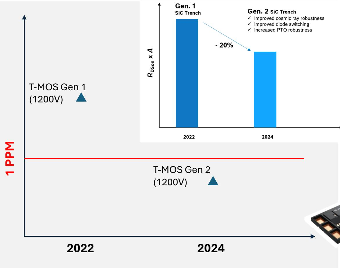
PPM rate calculation for an eight-chip module shows that a 2nd generation Bosch SiC MOSFET achieves less than 1 PPM failure rate related to cosmic radiation with 20% better  $R_{DS,ON} \times A$
