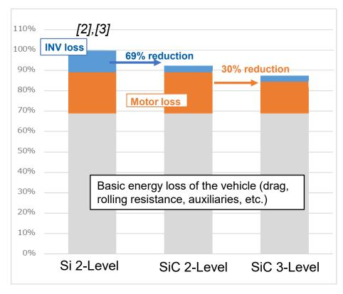
Real world tests show the previously studied loss reduction clearly. For reference, the change from Si to SiC gave BEV an approximate increase in efficiency by 7%. A similar result is expected with the change from 2 to 3-level inverters.
